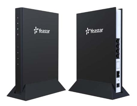
Yeastar TA Analogue VoIP Gateways are cutting-edge products that connect legacy telephones, fax machines and PBX systems with IP telephony networks and IP-based PBX systems.
